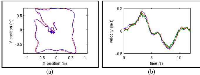
Figure 6: (a) Comparison between the position estimated by the onboard sensors (green) with ground truth measurements (blue). (b) Comparison of the ground truth velocity (blue) with the estimate from the EKF before (green) and after (red) optimization.
