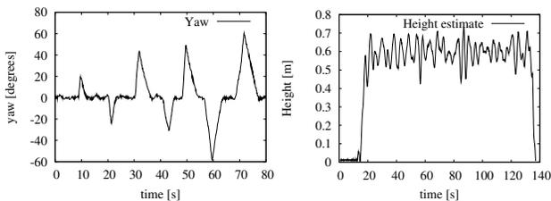
Fig. 6. Experiments for the autonomous stabilization of yaw (left) and height (right). During the yaw stabilization experiment, the quadrotor was required to rotate to  $0^\circ$ . From time to time, the user manually changed the yaw. After the user released the remote control, the quadrotor autonomously rotated back to the desired yaw angle. During the height experiment (right) the quadrotor was required to maintain height of 60 cm. The resulting error in height was  $\pm 10$  cm.
