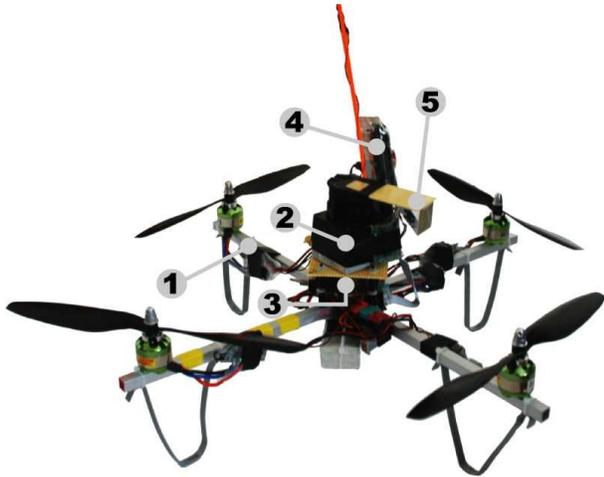
Fig. 2. The quadrotor platform used to evaluate the navigation system includes a Mikrokoopter (1), Hokuyo laser range finder (2), an XSens IMU (3), a Gumstix computer (4), and a laser mirror (5).
